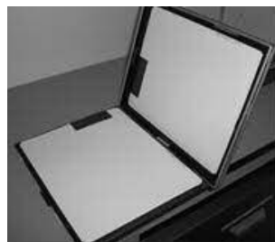
Figure 17: Intensifying screens inside a cassette
