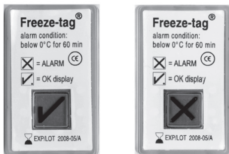
Figure 41.4 - Indicateur de congélation (Freeze-tag®)
